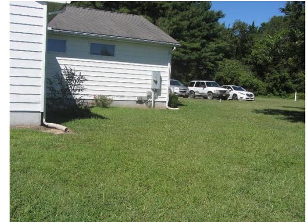
Stormwater currently drains from the property to the roadway. Parking spots in front of the building can be replaced with porous asphalt to capture and infiltrate stormwater and roof runoff. Rain gardens adjacent to the rear side of the building can capture, treat, and infiltrate additional roof runoff. A preliminary soil assessment suggests that the soils have suitable drainage characteristics for green infrastructure.
