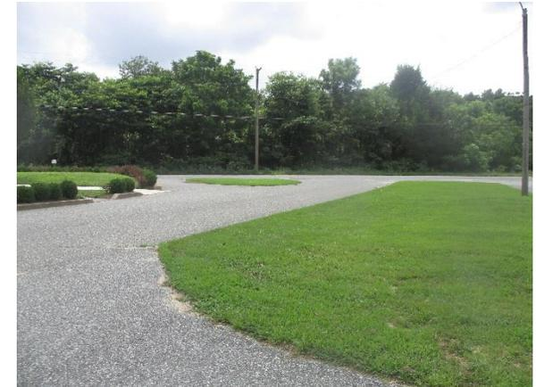
Stormwater currently drains from the property to the roadway. A bioswale placed on the east side of the island in the middle of the parking lot can capture, treat, and infiltrate roof runoff and stormwater runoff from a good portion of the parking lot. A preliminary soil assessment suggests that the soils have suitable drainage characteristics for green infrastructure.
